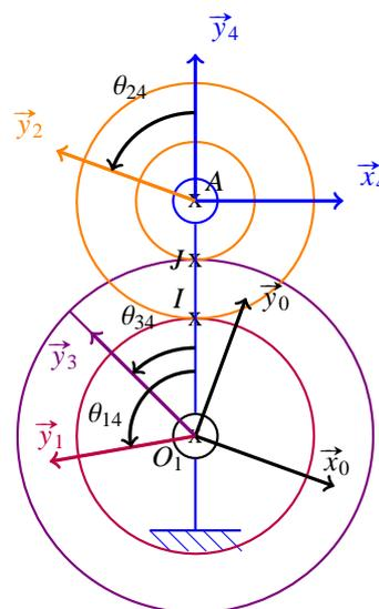
$$\lambda = \frac{\omega_{30} - \omega_{40}}{\omega_{10} - \omega_{40}} = (-1)^n \cdot \frac{Z_1}{Z_{2a}} \cdot \frac{Z_{2b}}{Z_3} \quad \text{ou} \quad \omega_{30} - \lambda \cdot \omega_{10} + (\lambda - 1) \cdot \omega_{40} = 0$$
