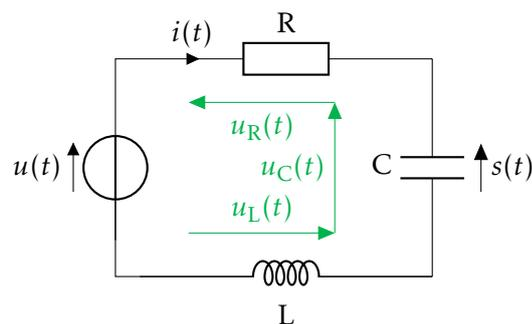
$$\begin{aligned} \Rightarrow u(t) &= u_R(t) + u_C(t) + u_L(t) \\ &= R \cdot i(t) + s(t) + L \cdot \frac{di}{dt} \end{aligned}$$
